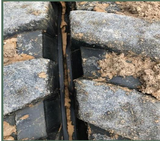
Especially when digging trenches, care must be taken to ensure that the entire load is distributed completely and as evenly as possible among the axles and tyres. This is because if, for example, the entire load acts on only one axle or even only one tyre, the total load can lead to serious tyre damage, as the photos below show.
